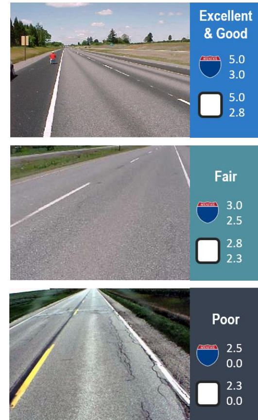
Figure 2.1 Pavement Serviceability Index
