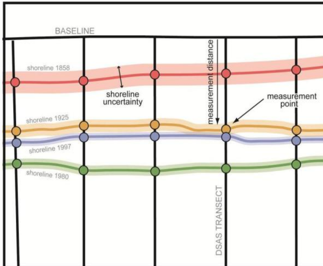
Figure 3-1. Diagram showing transects, shoreline measurement points, and positional uncertainty determined for the Massachusetts Shoreline Change Project.
