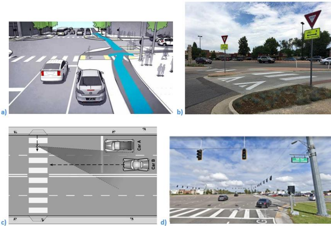
Figure 32. Illustrations of different geometric designs at intersections and crosswalks: a) protected intersection, b) raised crosswalk, c) near-side traffic signals, and d) advance stop line.
