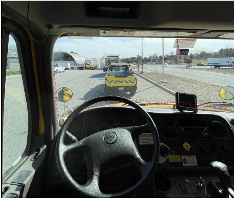
Figure 49. Image at 0 degrees where the right side of driver A pillar to midway across front hood is annotated.
