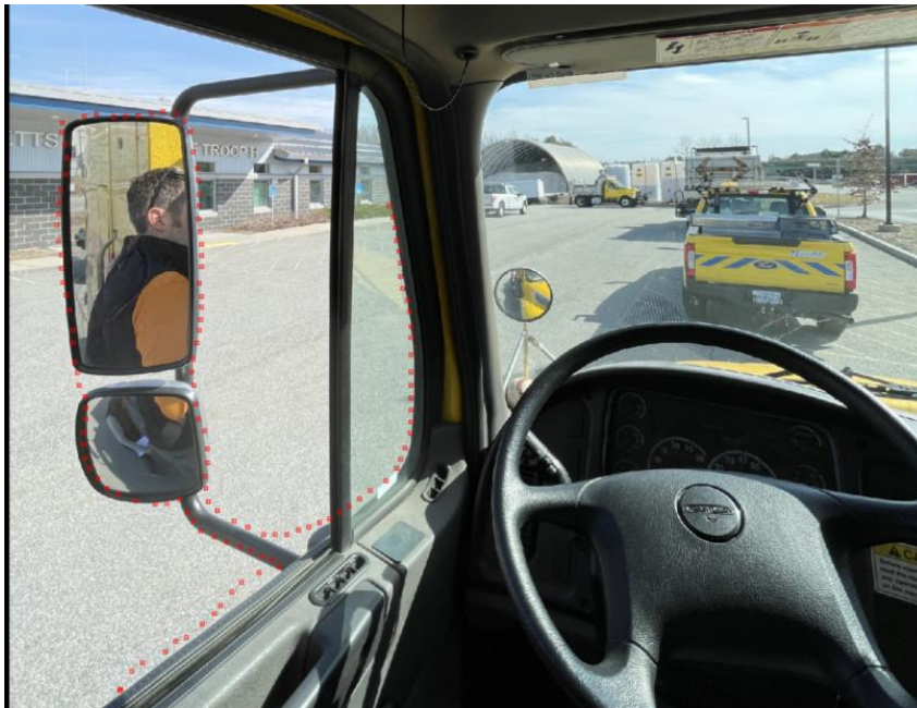
Figure 50. Image at -30 degrees where the left side of driver a pillar plus mirror is annotated.
