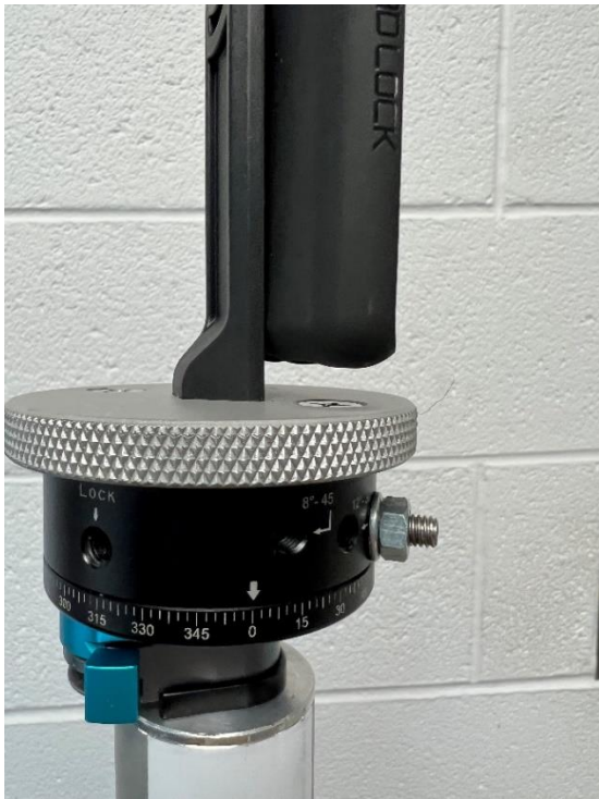
Figure 47. Rig shown at close range to show the method to rotate and line up the phone into the rig.
