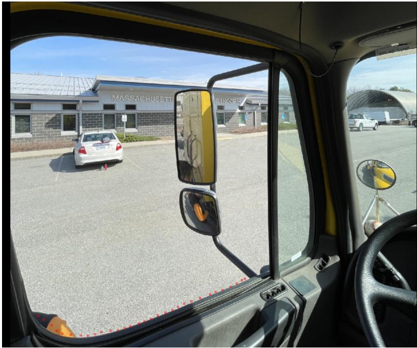
Figure 51. Image at -60 degrees where the annotation finishes the rest of driver window. Note that this may need to go to -90 or -120 degrees for some vehicles.
