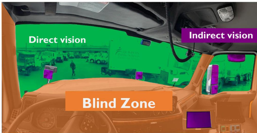
Figure 1: View from the driver's seat of an International HV 513. Direct vision of the environment is shaded green (unobstructed view through the windows), indirect vision areas are shaded purple (mirrors and camera display unit), and the blind zone areas are shaded in orange (hood, A and B pillars, and door).
