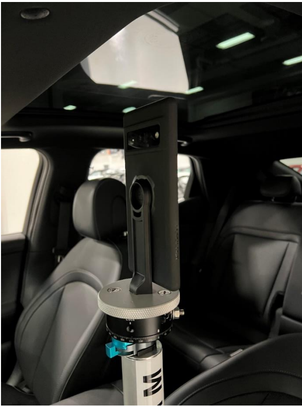
Figure 43. Close-up of rig with phone installed for measurement.
