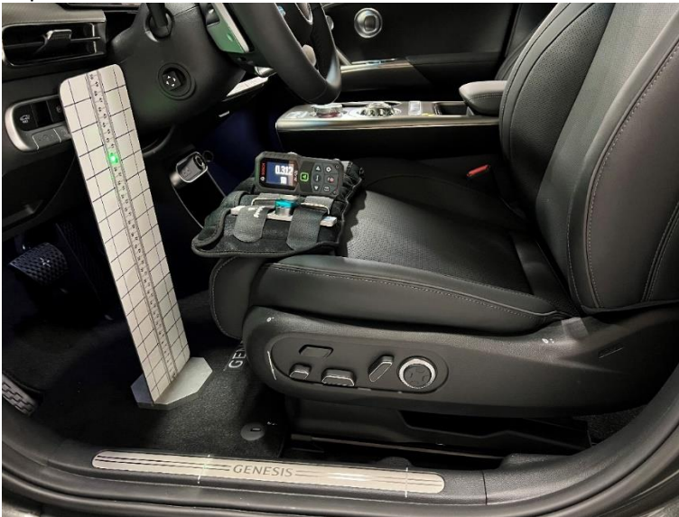
Figure 40. Laser being used to identify the exact mid-point for seat, which will be used for rig placement and data collection.
