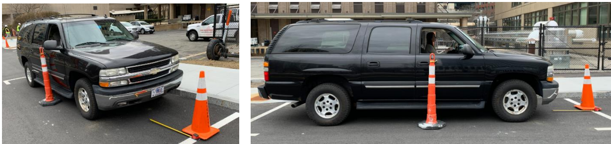
Figure 31. Setup for 3-foot and 4-foot cone method of blind zone measurement.
