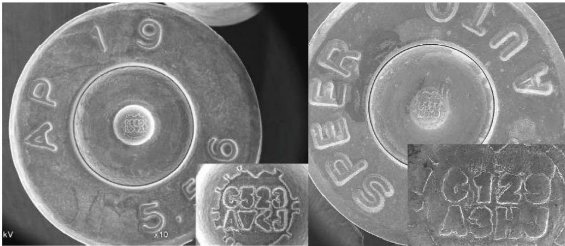
A 5.56x45 mm cartridge fired from a AR-15 rifle after 341 rounds of firing (left), and a 45 caliber cartridge fired from a semiautomatic pistol after 8,532 rounds of firing (right).
