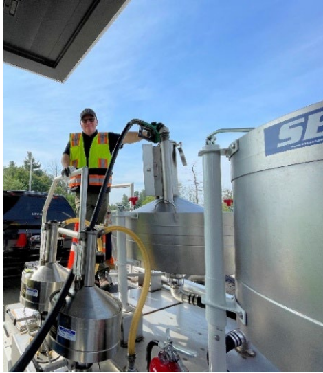
Compliance Officer David Holden using a propane prover to test the meter on a propane delivery truck to ensure that the truck will deliver the amount of propane for which it charges the customer.
